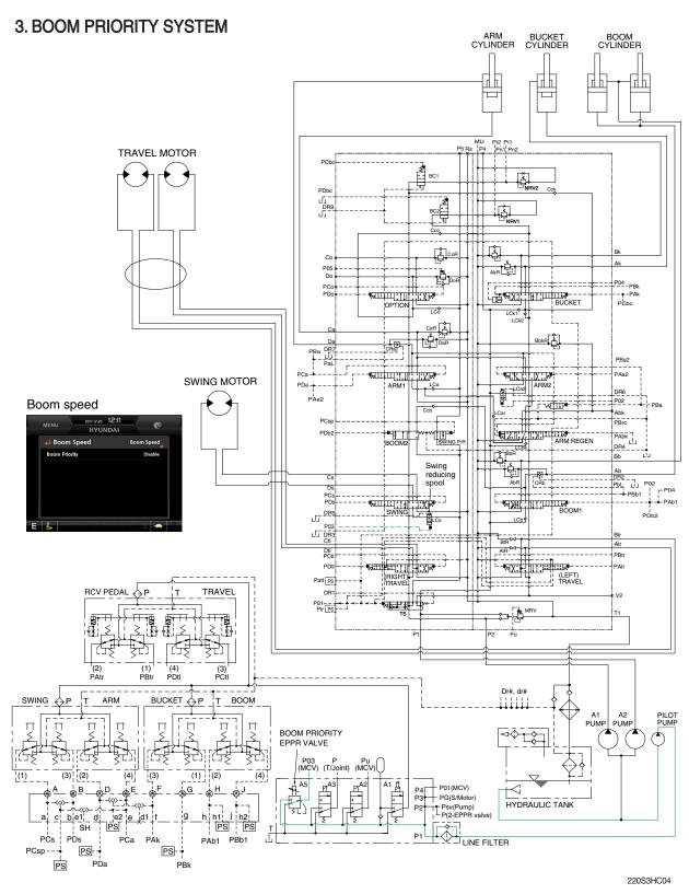
When carrying out the combined operation of swing and boom up, the boom up operating speed is lowered then normal operation.
